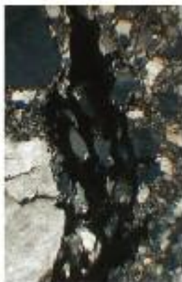
Fig. 9. Stöttham diamictite: photomicrograph of a sandstone sample containing glass from probable shock melt – black under crossed polarisers of the microscope. Field width 1.6 mm.
