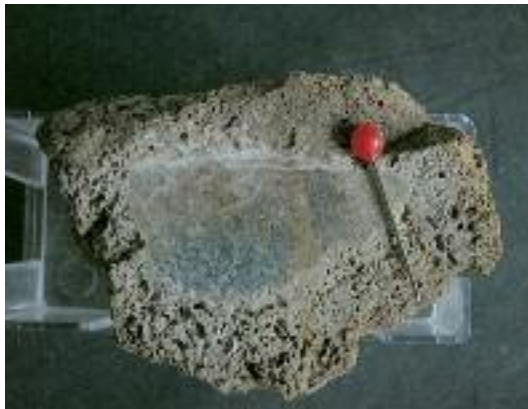
Fig. 8. From the Stöttham impact layer: sawed surface of a silica limestone exposed to strong heating. Only a core has retained its original texture. In the outer zone the carbonate has disappeared by decarbonisation and/or melting.
