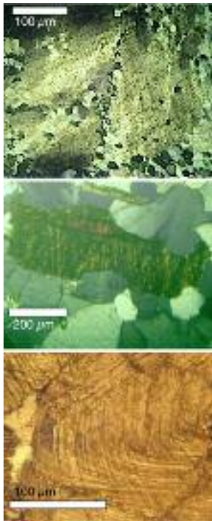
Fig. 18. Typical shock effects as identified in rocks from the Lake Tüttensee impact layer. Top down: Planar deformation features (PDFs) in two quartz grains; two crossing sets of kink bands in mica; multiple sets of plastically deformed microtwins in calcite.
